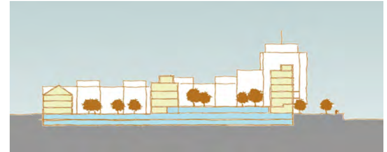
Option 2, Cross Section BB (Note two underground levels and one ground floor level providing a podium above which a central landscaped courtyard could be provided)
