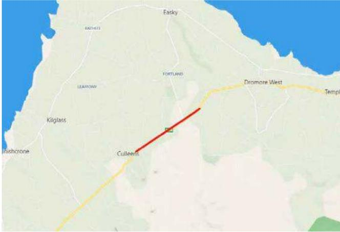
The N59 Owenbeg Phase 3 which runs from Camcuill to Culleens involves structural rehabilitation and strengthening of 4km recycling of the existing N59. The works will take place in bog rampart and will include recycling of the existing pavement and resurfacing with SMA.
