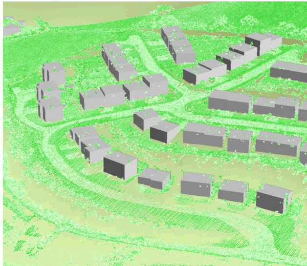
Figure 6-4: Sample Point Cloud from Aerial LiDAR Survey
